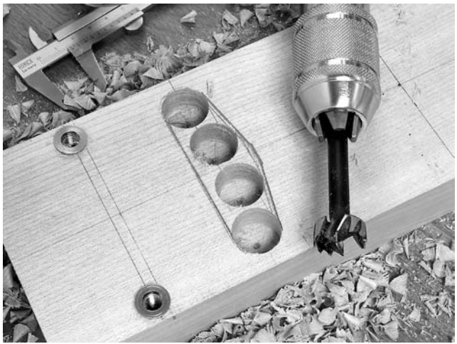
The pre-drilled pickup cavity
