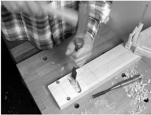
Removing the remaining material with a chisel
