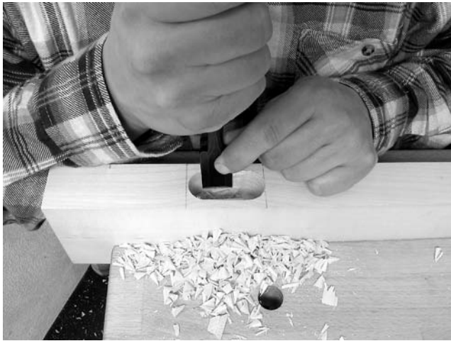
Cleaning up the cavity
